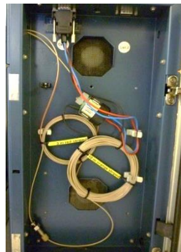
Figure 1. PQ tubing kit installed in detector oven and connected to flow cell.
